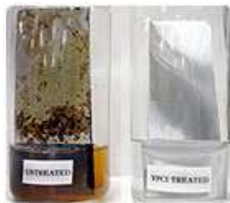
Corrosion .Coupon Study Left: Without VpCI Right With VpCI
