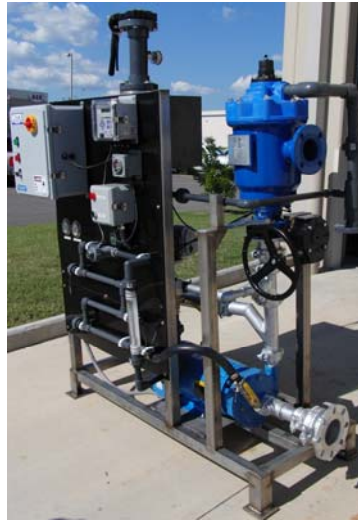
Figure 2. A Standard VRTX Unit with a Separator System and Controls
