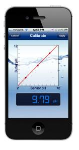
Allows for calibration with any number of pH buffers
