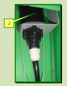
\*Patented Dual-Valve Overflow Safety System: Should the primary solenoid valve remain stuck in the open position or if a leak-by occurs, the secondary float will activate, closing the overflow solenoid valve. (Non-powered magnetic mechanical solenoid valves)
