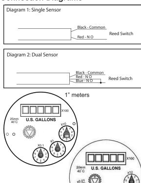
ring. With fingers, lift the magnet pointer off its shaft and remove the plain pointer from the target dial. Reverse their positions and press them firmly into place. Securely seat the sealing ring and then replace the lens, matching the tab on the lens to the notch on the meter so as to align the sensor with the magnetic pointer dial. Thread the meter top on and tighten.
