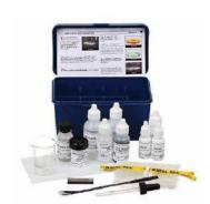
Boiler deposits can result from improper product application, lack of blow down, softener failure, low alkalinity, iron contamination, return line corrosion byproducts or process contamination. The deposits test kit is a quick and easy way to point the water treatment engineer in the right direction for problem solving. This kit is designed to be an onsite help and is not intended to replace full laboratory analysis of the deposit.
