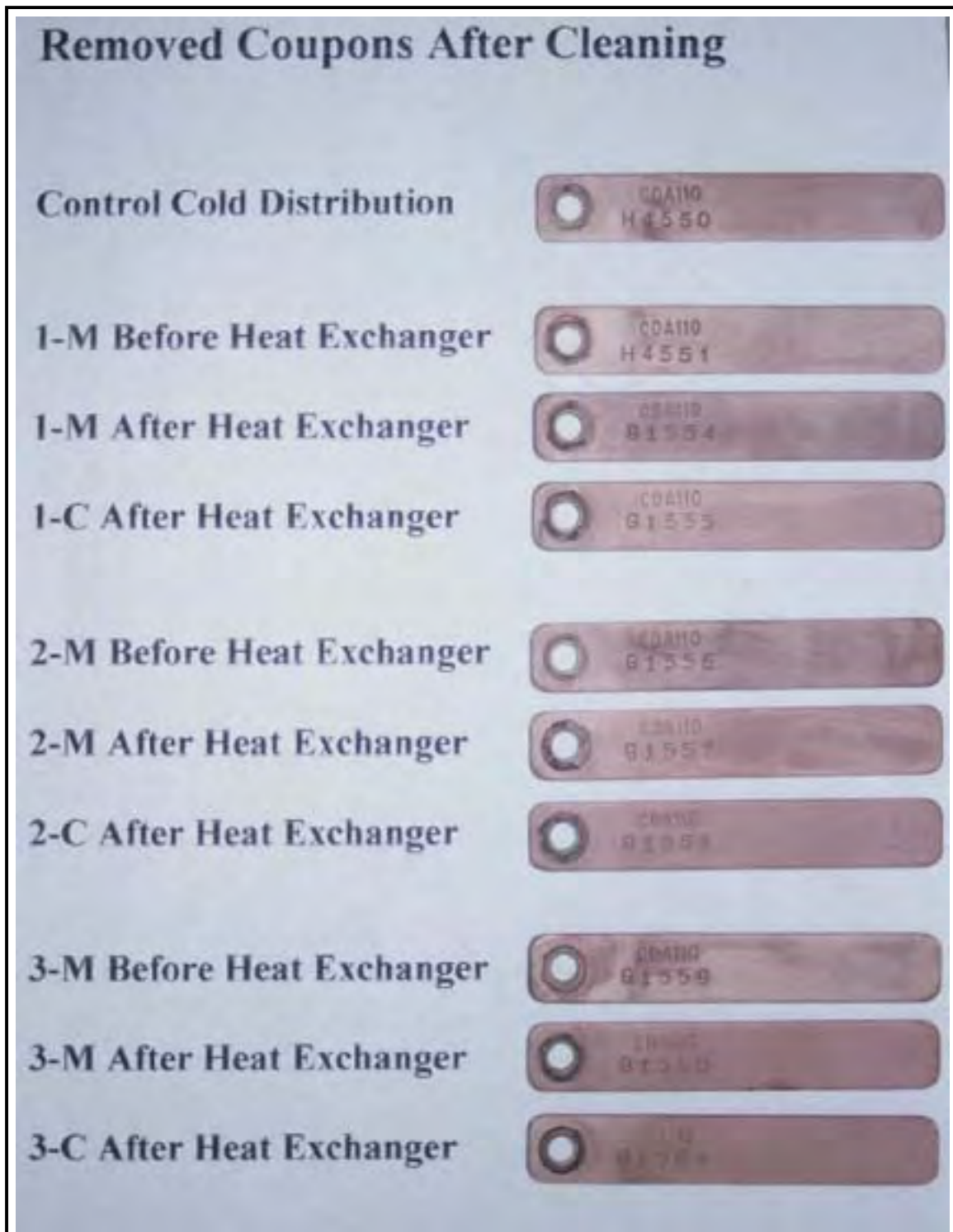
Figure 8. Corrosion coupons after cleaning.
