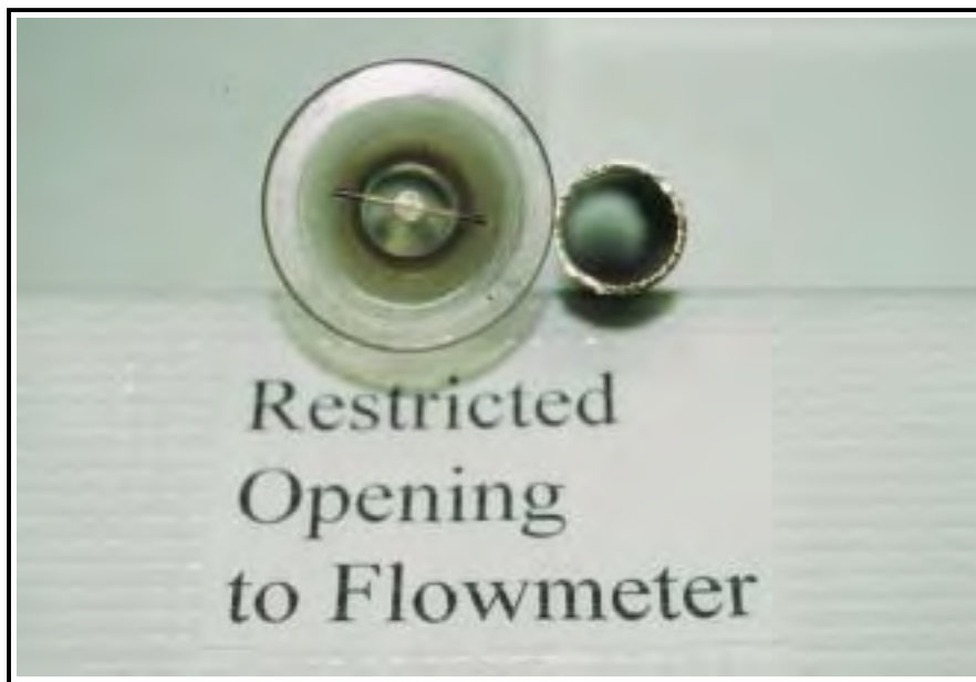
Figure 9. Restricted opening — flowmeter.
